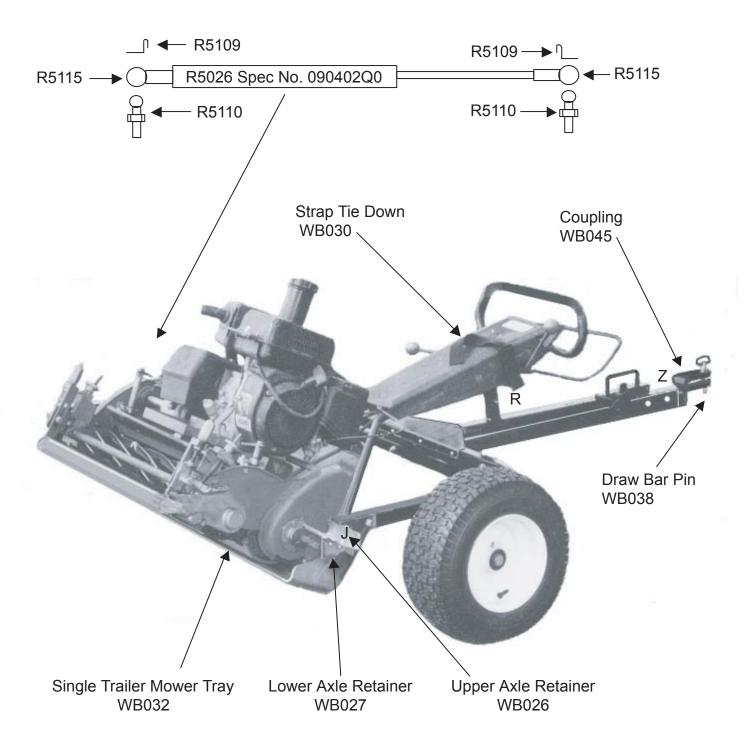
Picture showing mower correctly positioned in tray WB032, with the axle located under the Upper Axle Retainer WB026 & inside Lower Axle Retainer WB027 then strapped in with WB030
